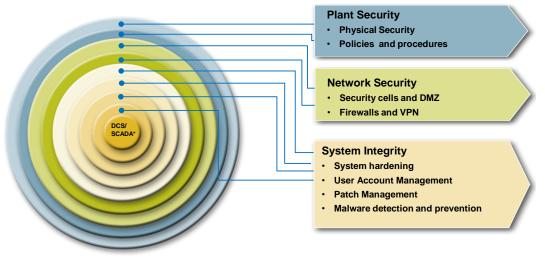
The advantage of this strategy is the fact that an attacker first has to break through several security mechanisms to do any damage. The security requirements of each layer can be taken into account individually.
